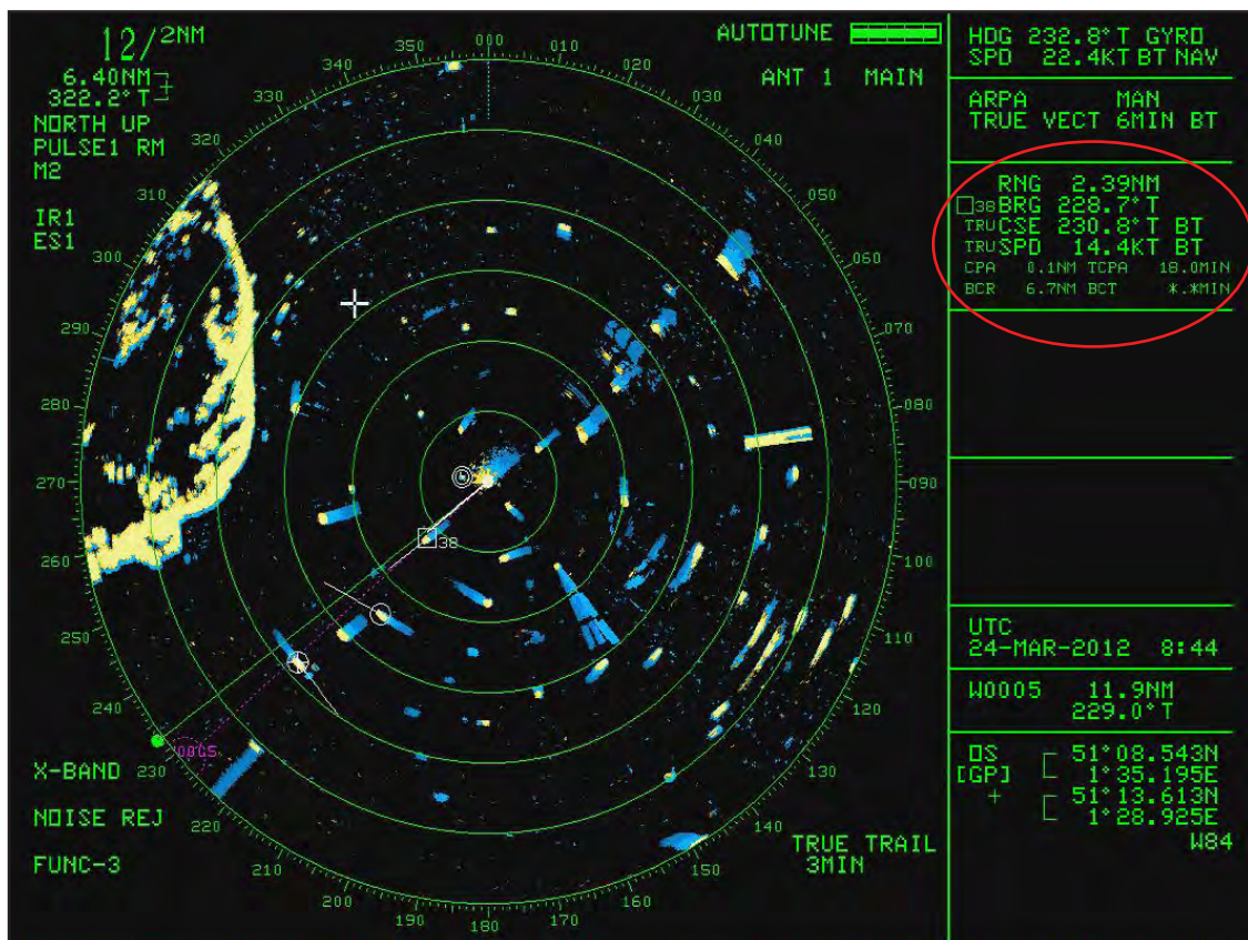
Figure 4: 0844 X-Band radar display showing data selected for one target
