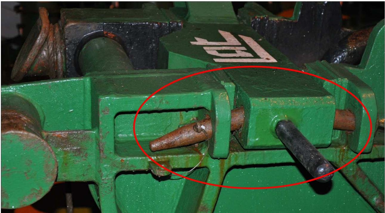
Figure 7: Bent chain stopper locking pin Source: DMAIB
