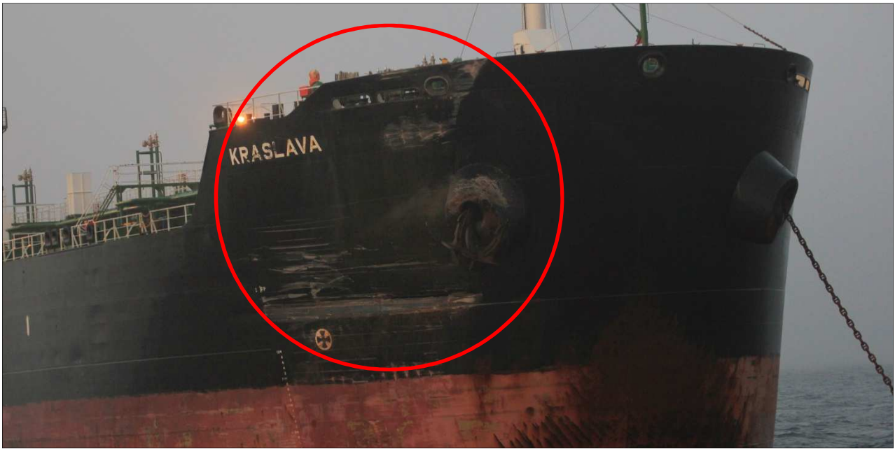
Figure 6: Damages on KRASLAVA Source: Danish Naval Home Guard
