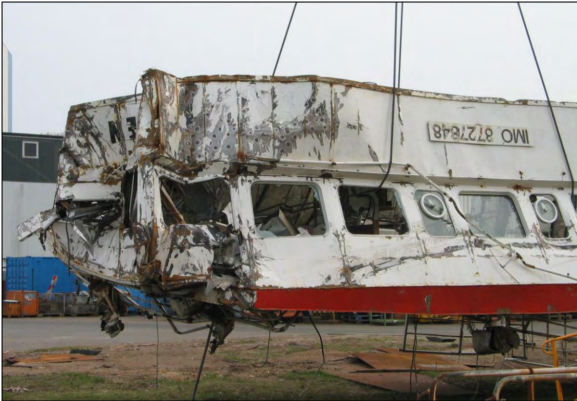
Figure 17: TYUMEN-2, point of impact on the port side front of the wheelhouse
