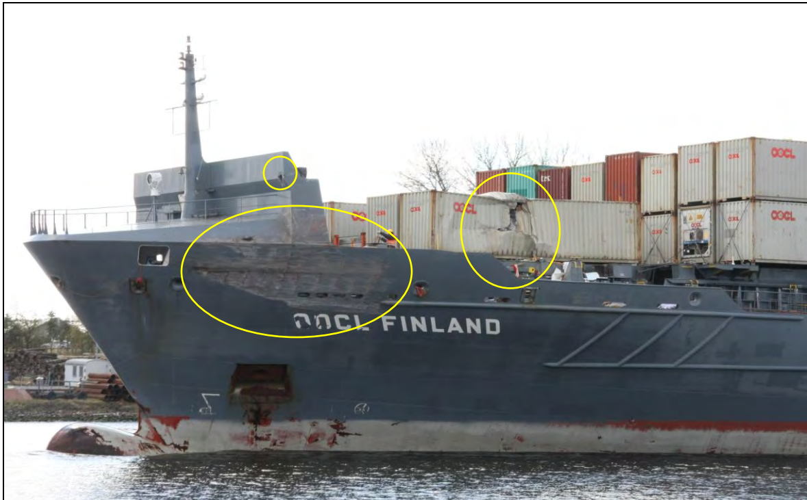
Figure 6: OOCL FINLAND, damage to the bow and one container
