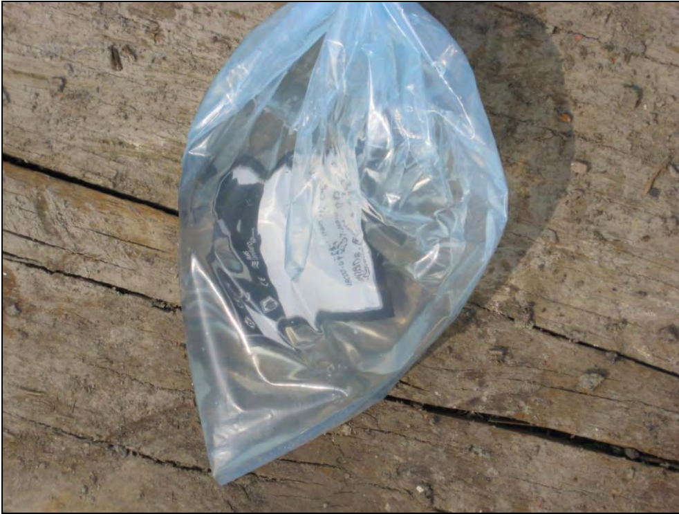
Figure 12: CompactFlash memory card from the voyage data recorder's central processing unit in the water-filled shipping bag
