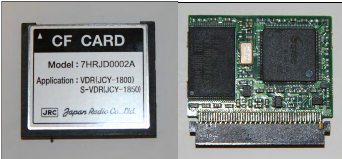
Figure 19: CompactFlash memory card; disassembled in the image to the right
