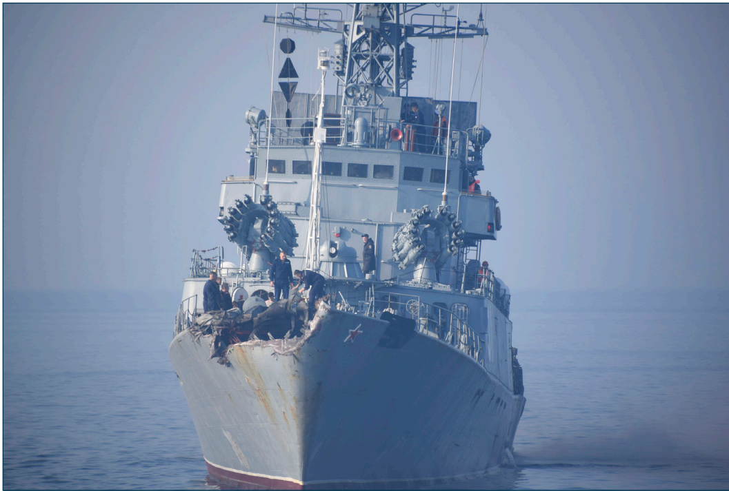
Figure 14: 311 KAZANETS' damages Source: Private photo
