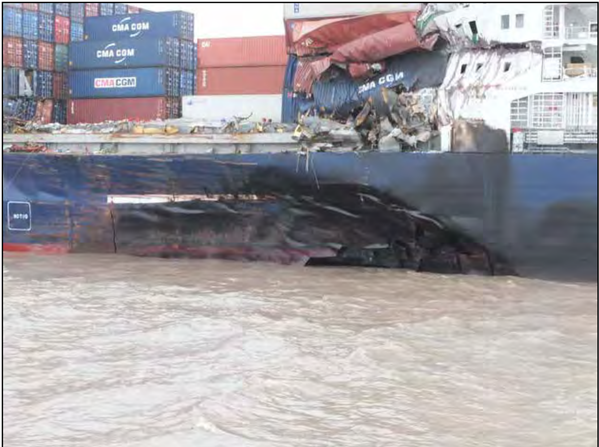
Figure 8: Close-up on CMA CGM Florida's damaged port side
