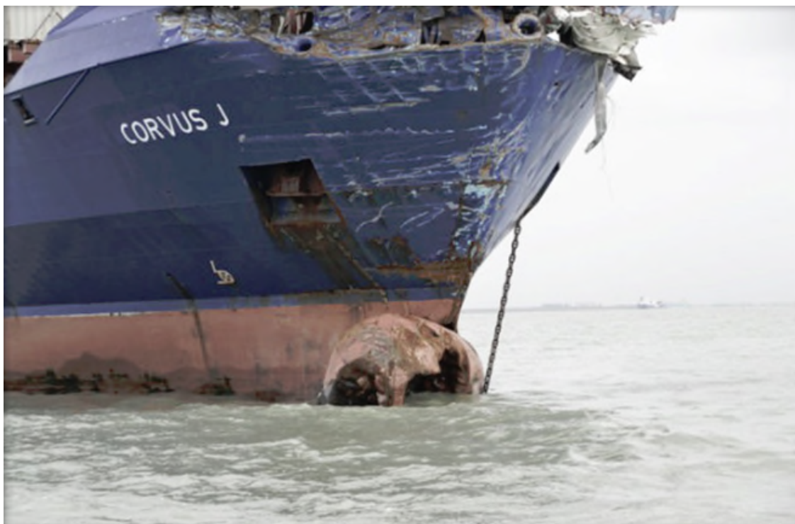
Figure 23: Bow damage to Corvus J post collision
