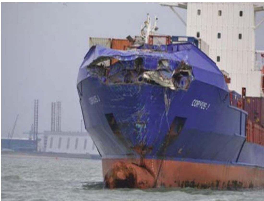
Figure 21: Bow damage to Corvus J post collision
