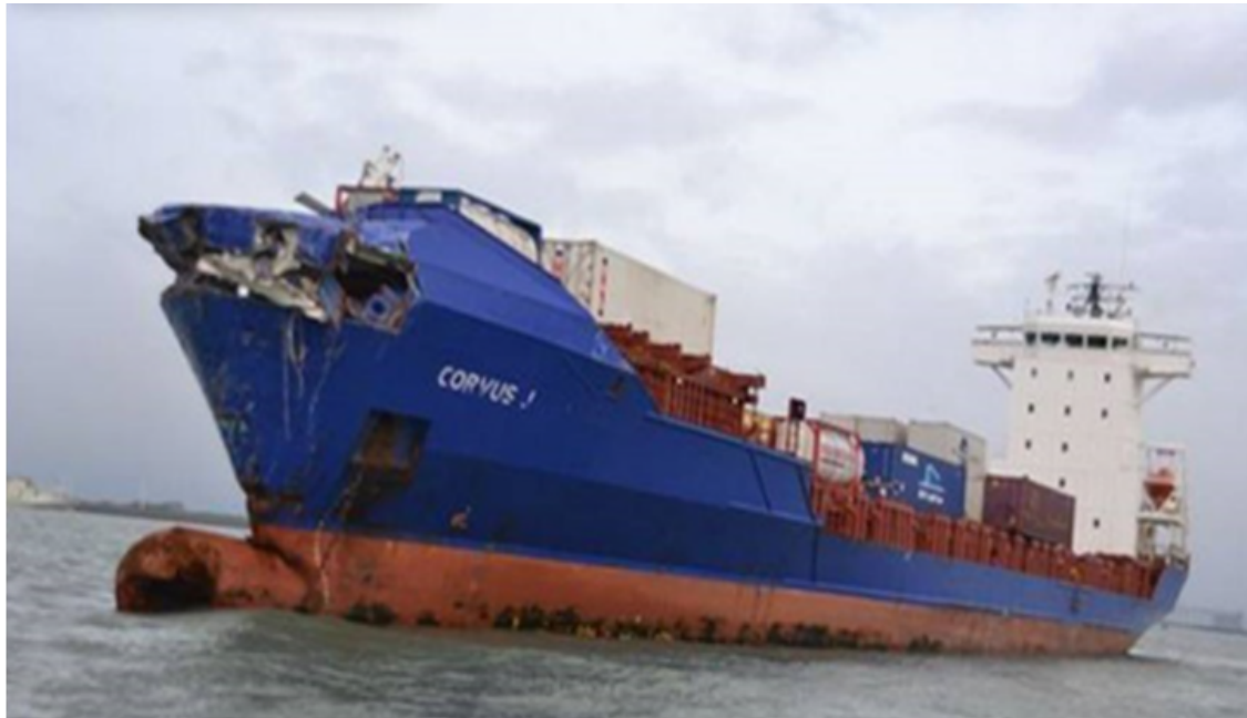
Figure 22: Port bow view of Corvus J post collision
