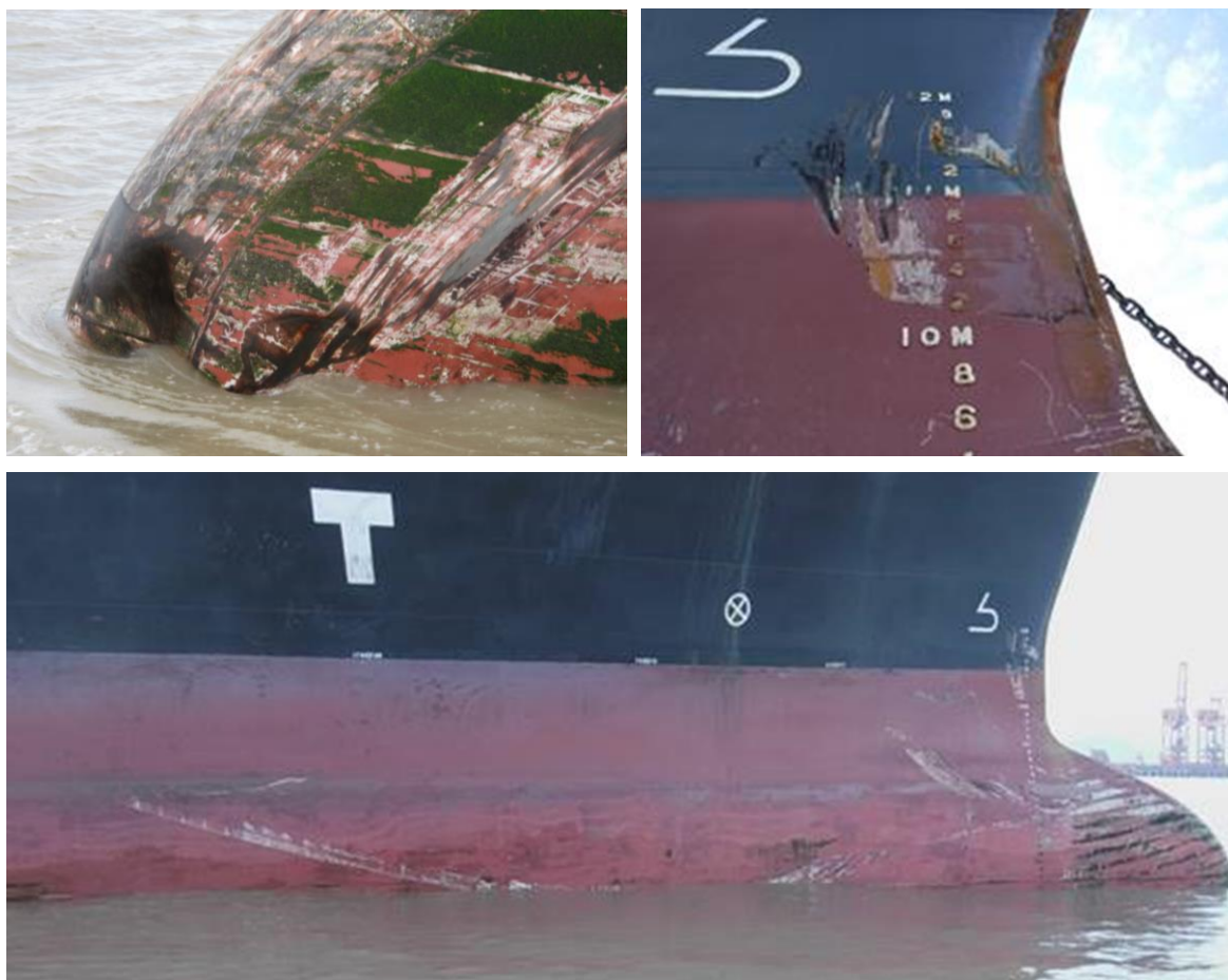
Figure 7: Polar Spirit, indentations on bulbous bow and starboard bow, scratches along the starboard side
