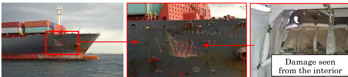
Photo 3 Damage to Vessel C
