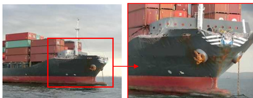
Photo 2 Damage to Vessel B
