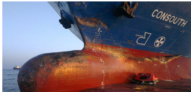
Figure 10. Consouth damaged port bow and her lifeboat used following the collision.
