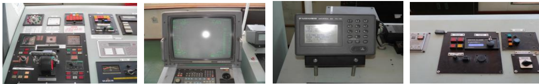
Figure 13. Consouth main bridge equipment. Main engine control lever, ARPA, AIS, BMWAS.
