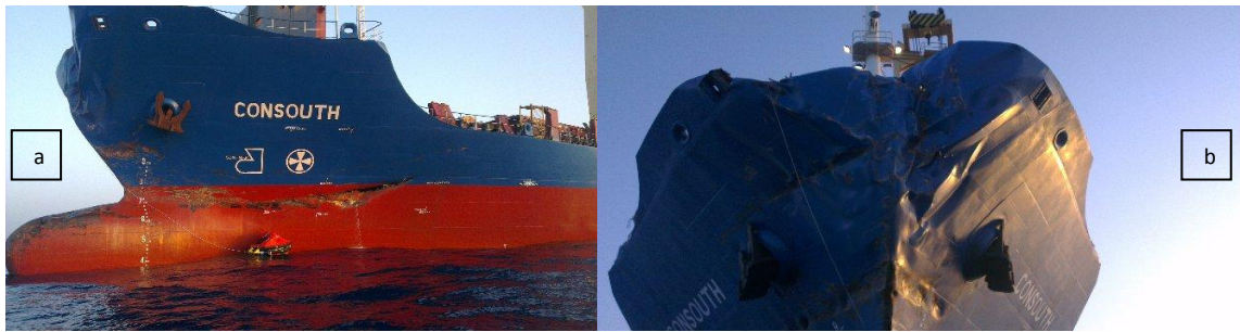
Figure 9.a.b. Consouth damaged morning hours on the day of the collision.
