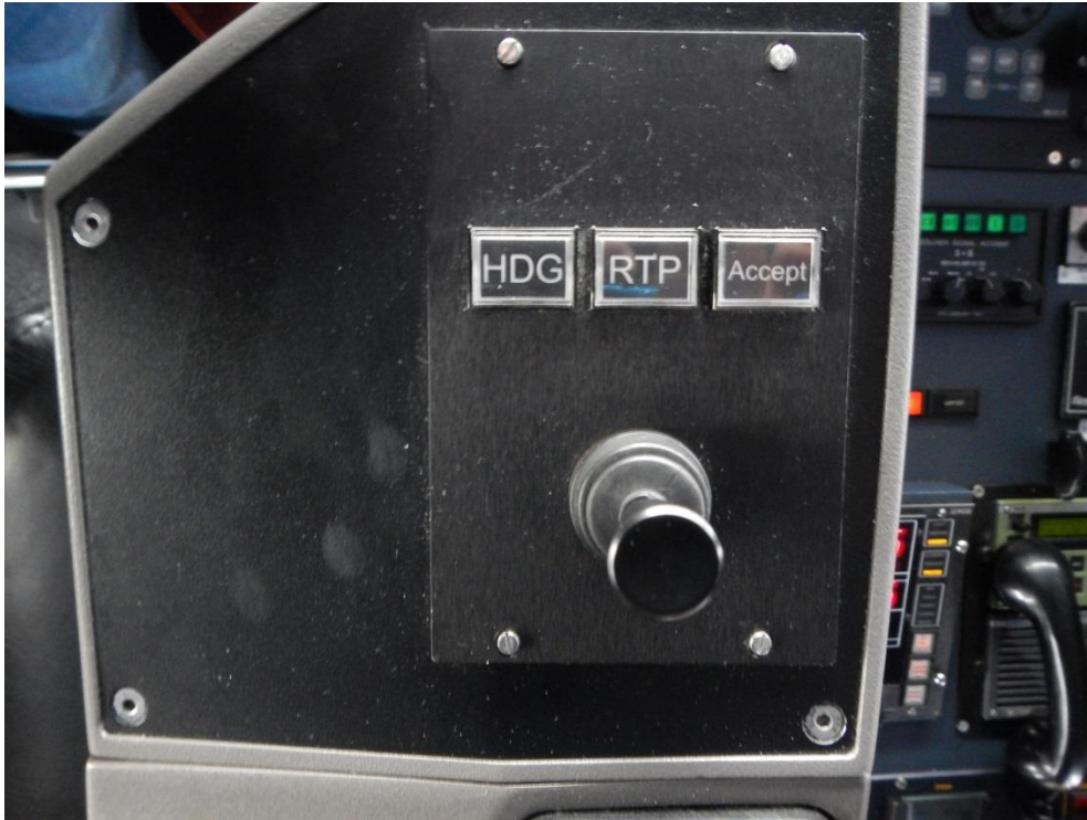
Fig. 9. The joystick for the automatic steering system that was used on STENA JUTLANDICA, located on the armrest of one of the navigator's chairs.
