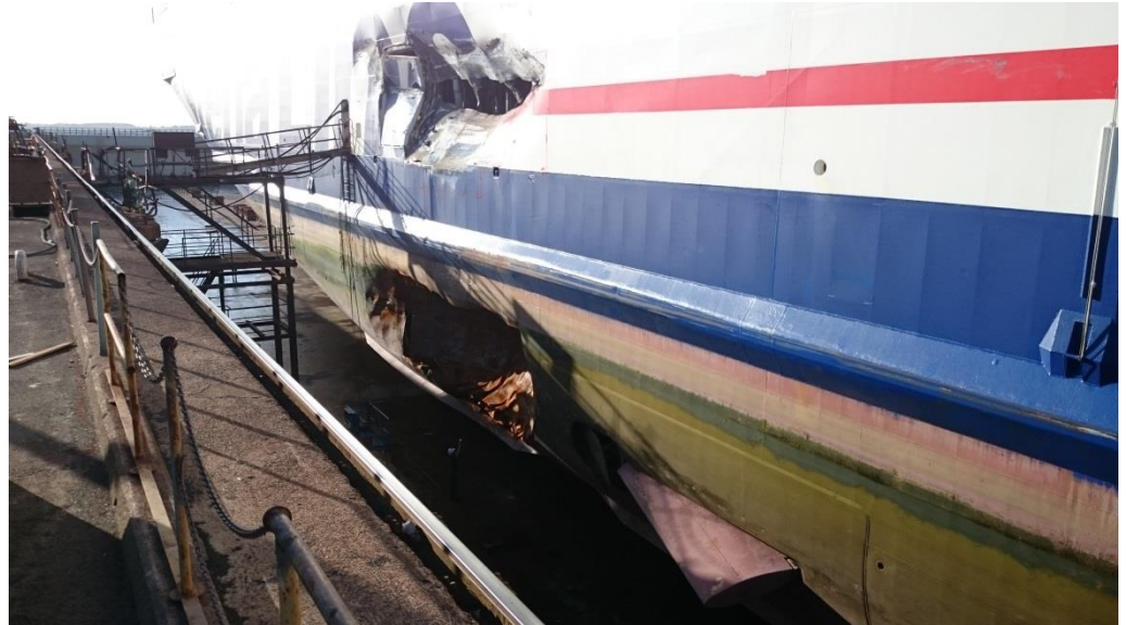
Fig. 5. Damage to STENA JUTLANDICA. The photograph is taken in dry dock. Image: Termtank.
