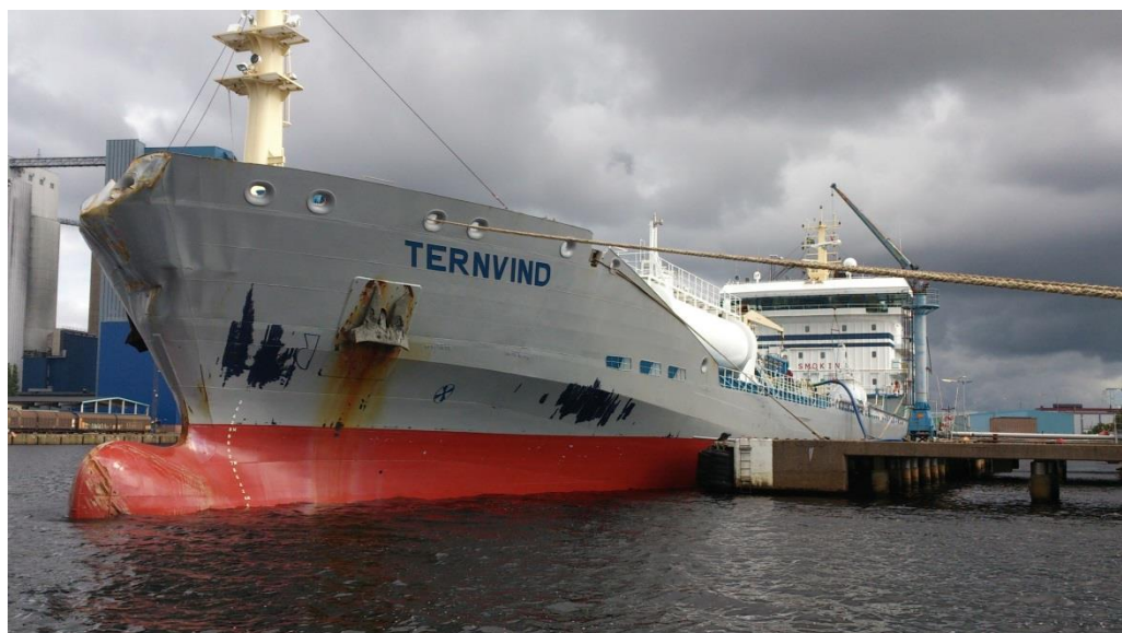
Fig. 6. Damage to TERNVIND.
