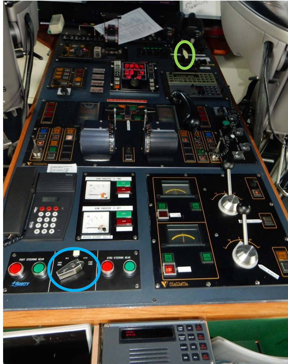
Fig. 10. The desk between the navigators' chairs on STENA JUTLANDICA. The override knob is located close to the officer's chair, circled in green (top right of the image). The knob to switch between different methods of steering the vessel is on the aft part of the panel, circled in blue (bottom left of the image).
