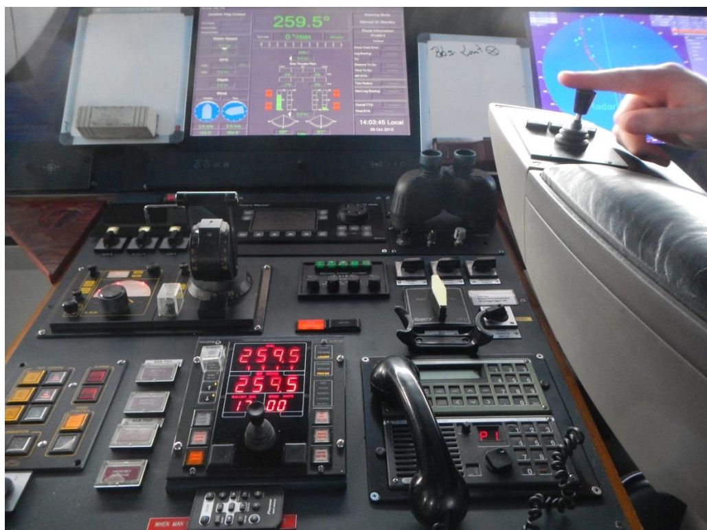
Fig. 8. The desk between the navigators' chairs on STENA JUTLANDICA. The knob that is used to override the steering can be seen marked with fluorescent tape on the right, between the binoculars and the VHF receiver (see also Fig. 10). The finger in the upper-right corner is resting on the joystick for the automatic steering system that was used on this occasion.
