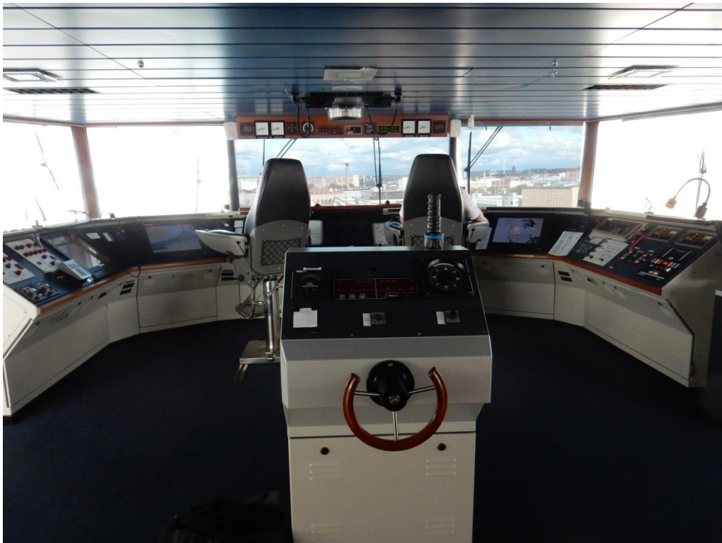
Fig. 7. The bridge on STENA JUTLANDICA. The desk where manual steering takes place is in the foreground, in the middle of the image. The rudder angle indicator is visible below deck (in the roof) between the chairs.
