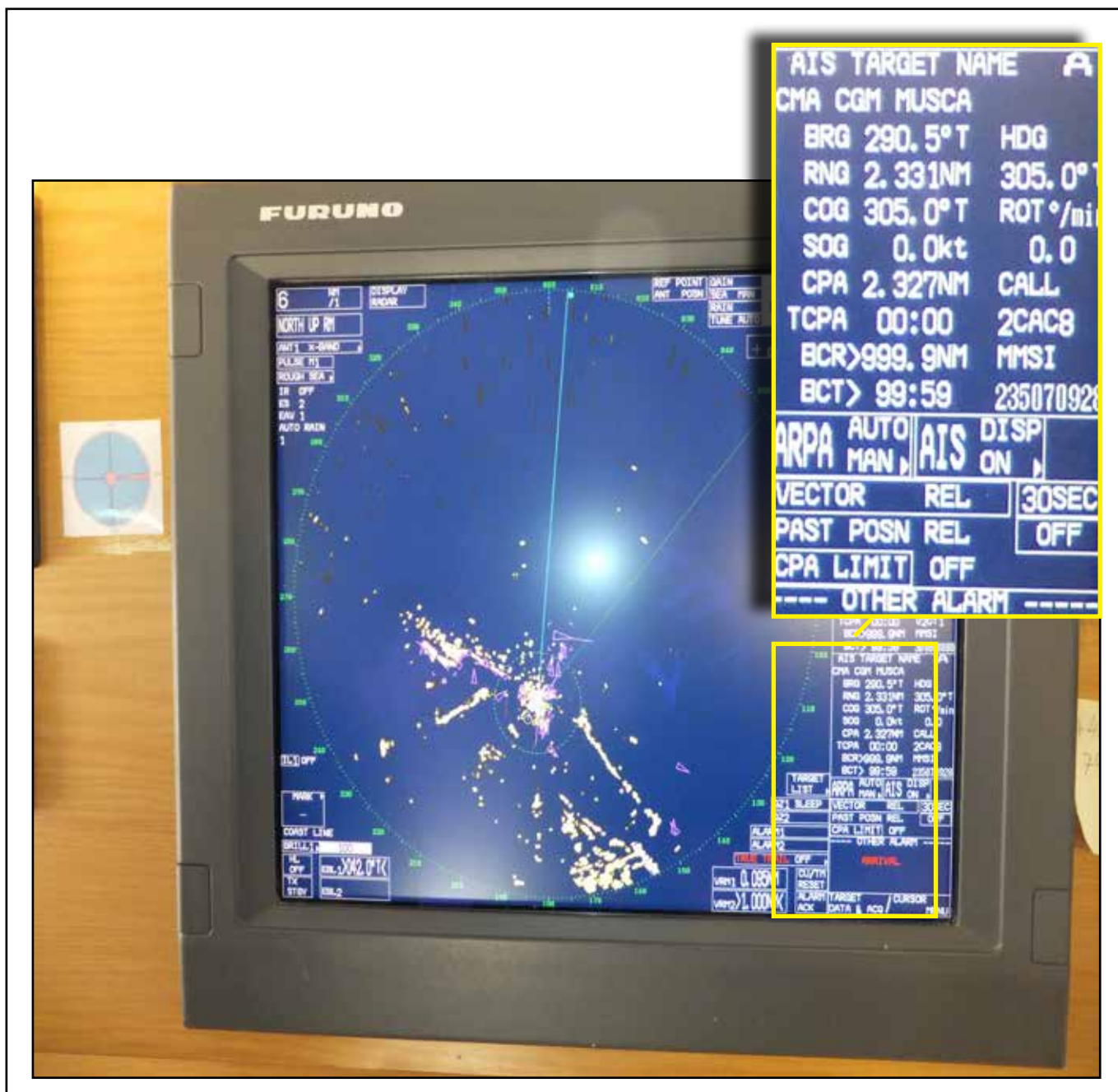
Figure 10: AIS information on Paula C 's port radar display
