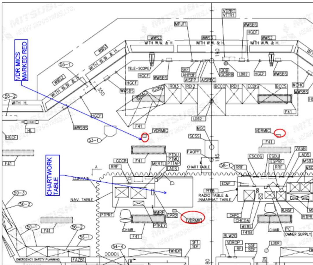
**Figure 2: Bridge layout, showing position of chartroom and VDR microphones (red)**
