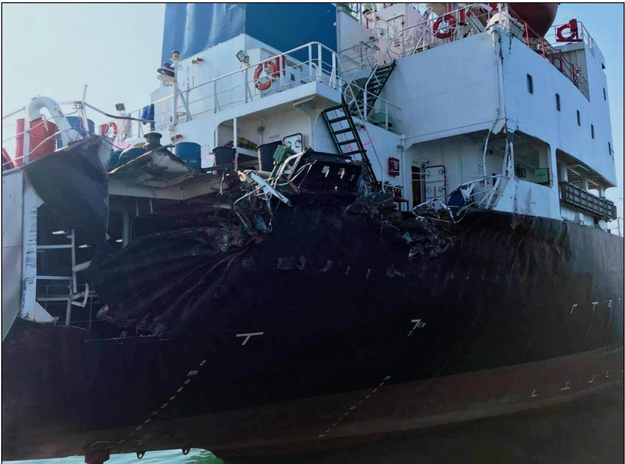
**Figure 3: Damages sustained by *DK Iman***
