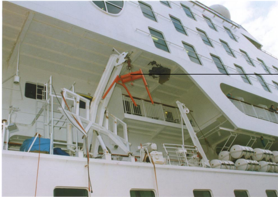
Davit & Lifting cradle of missing No. 1 Lifeboat
