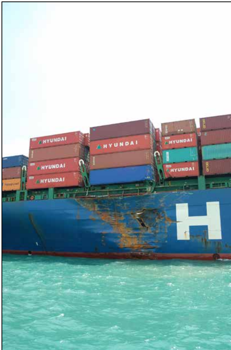
Figure 11: Damage to Hyundai Discovery 's port side No. 2 water ballast tank
