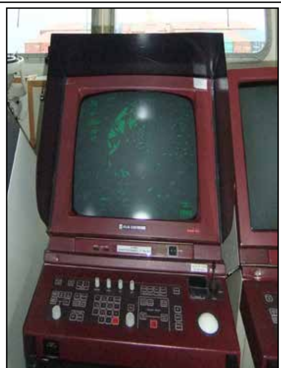
Figure 16b: Hyundai Discovery's starboard side S band radar
