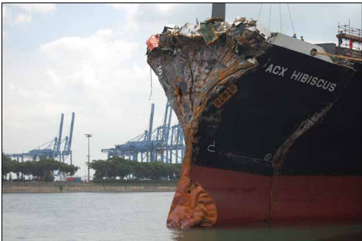
Figure 10: Damage to ACX Hibiscus's bow
