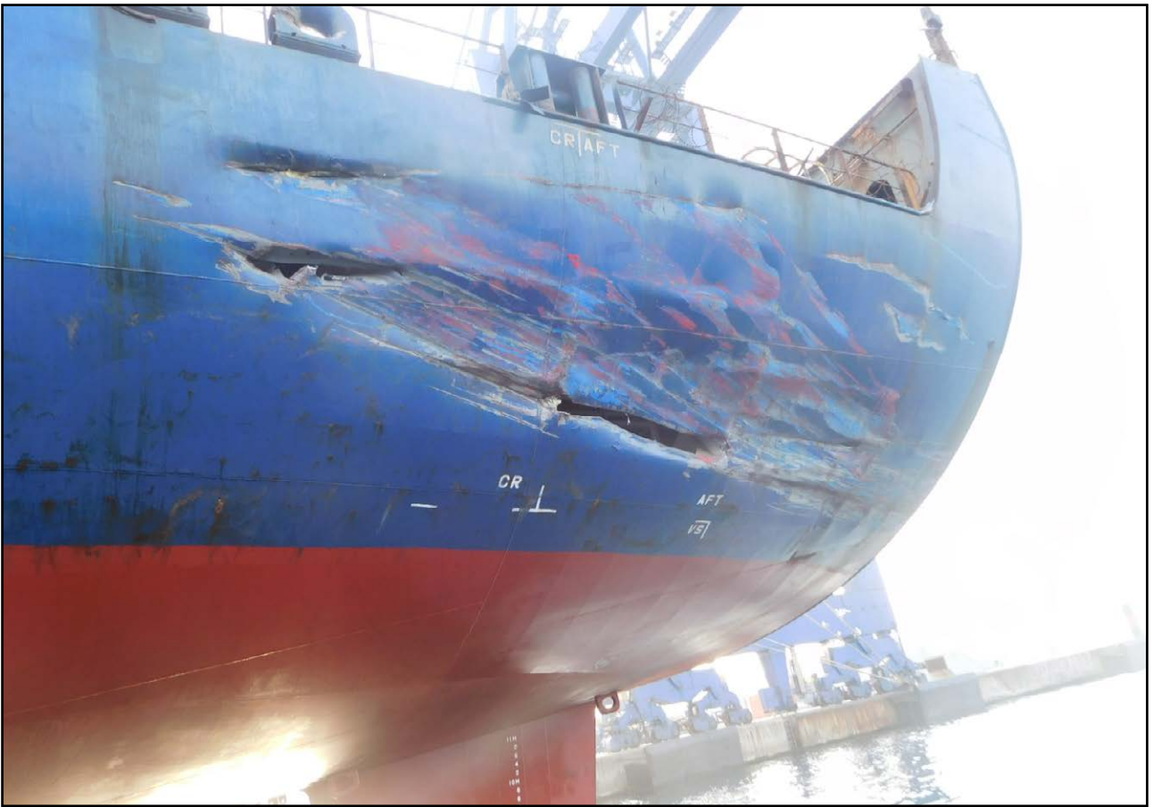
Figure 11: Detail of damage to ANL Wyong's port quarter
