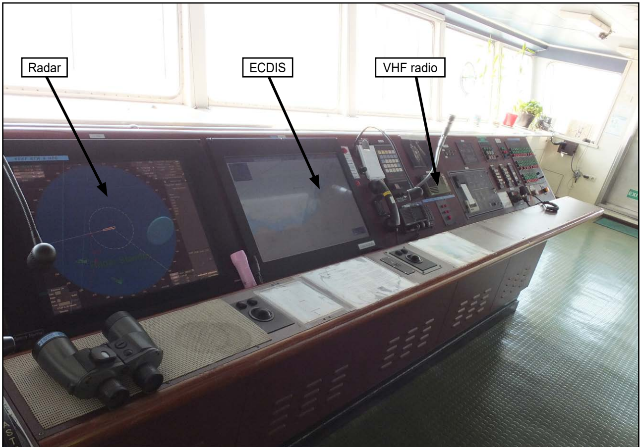
Figure 4: The starboard side of ANL Wyong's bridge console showing the radar and ECDIS displays in use by the OOW
