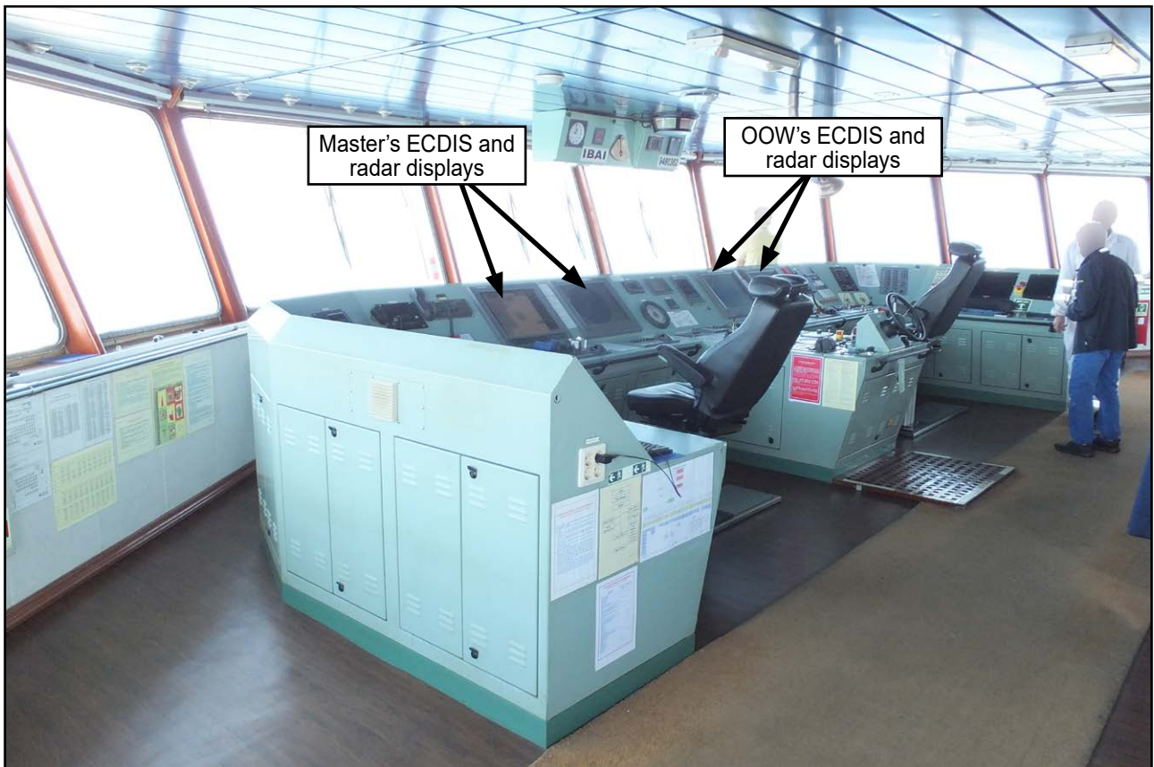
Figure 5: King Arthur's bridge horseshoe arrangement showing the displays in use by the master and OOW
