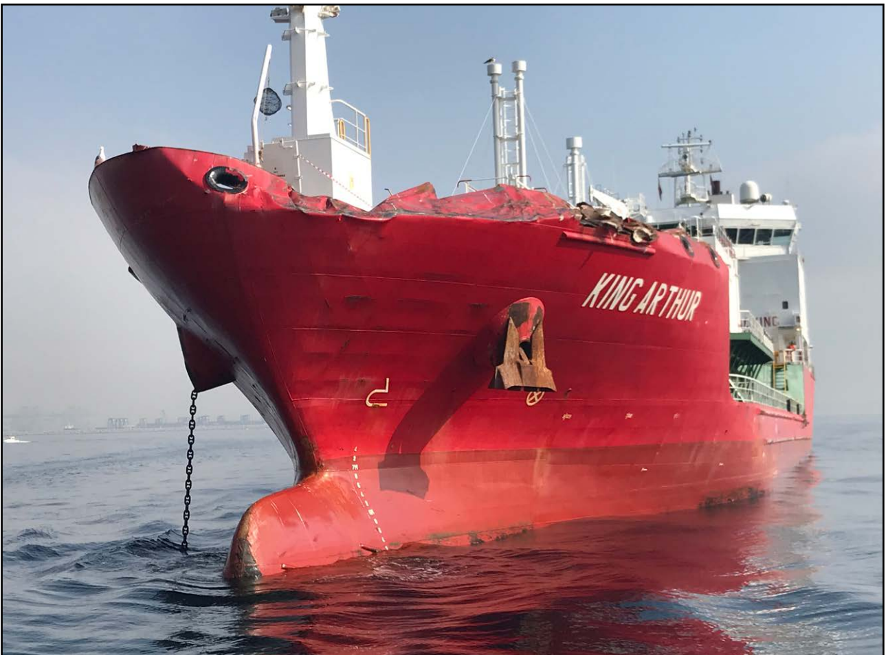
Figure 12: Detail of damage to King Arthur's port bow
