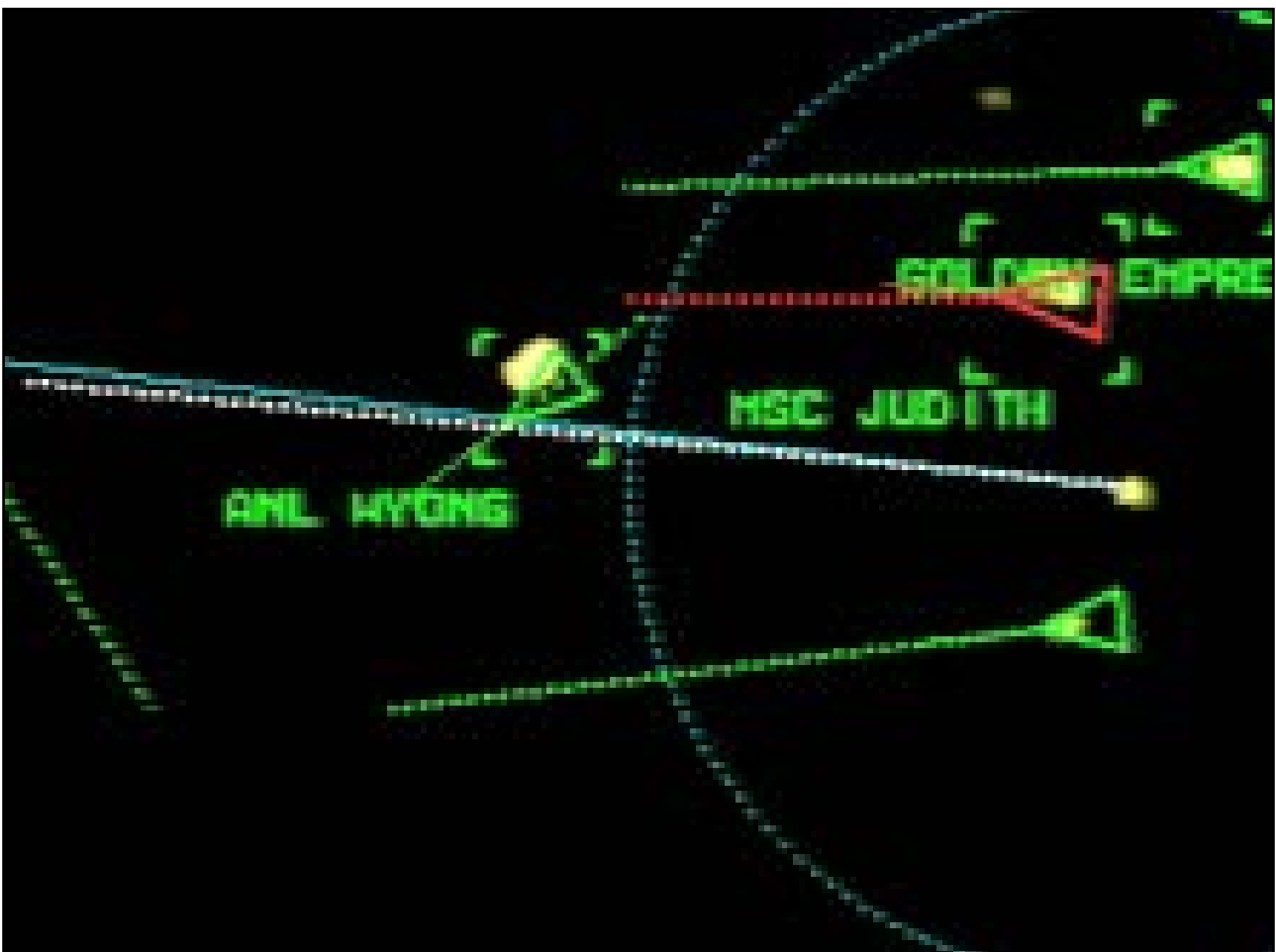
Figure 17: Detail from King Arthur 's starboard radar display showing the AIS symbol for ANL Wyong heading in a south-westerly direction
